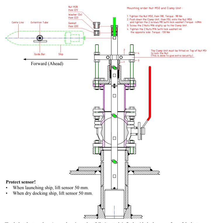
Check that the transducer/sensor housing, when fully inserted, is flush with the lower surface of the bottom flange.
