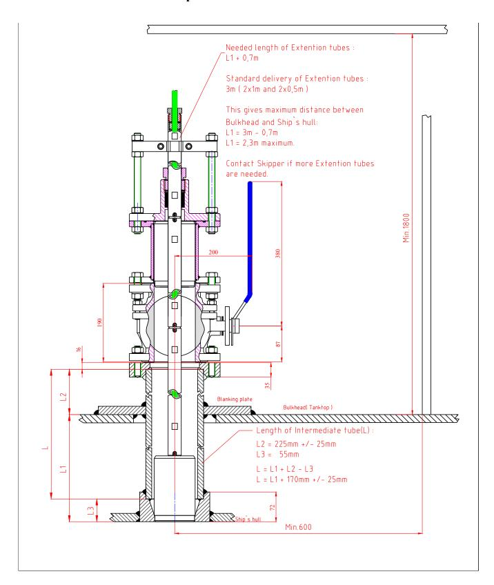
The Sea Valve should be placed in a service accessible place large enough for installation and disassembly of the transducer/sensor unit.
